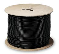
CAT 6 outdoor network cable, F/UTP type with black PE sheath, shielded with aluminum foil, 305-meter spool, composed of 4 balanced 100 Ohm pairs with flexible AWG 23 red copper conductors.
